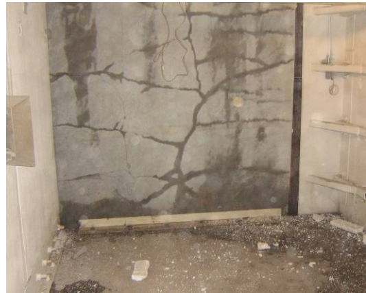
Figure 26: Internal view of CFRP panel after Experiment 5
