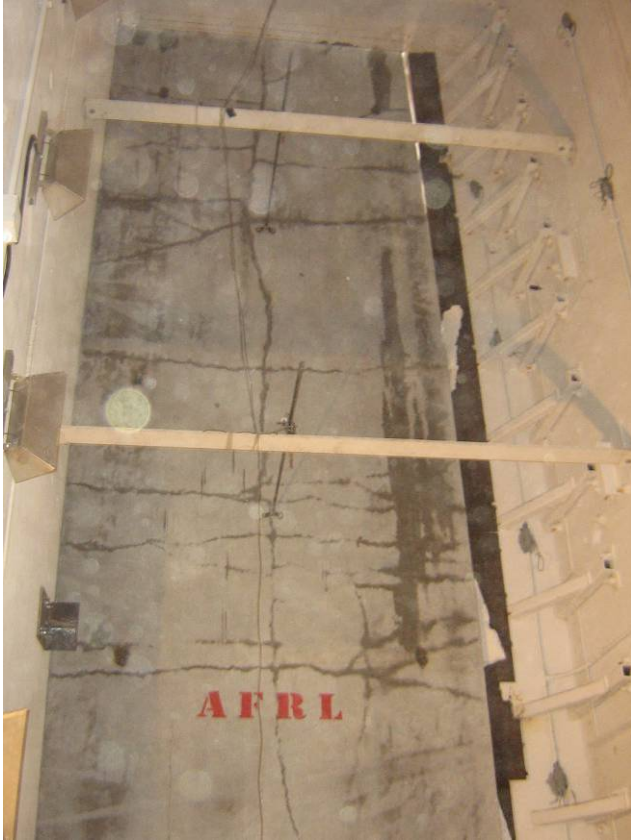
Figure 26: Internal view of CFRP panel after Experiment 5
