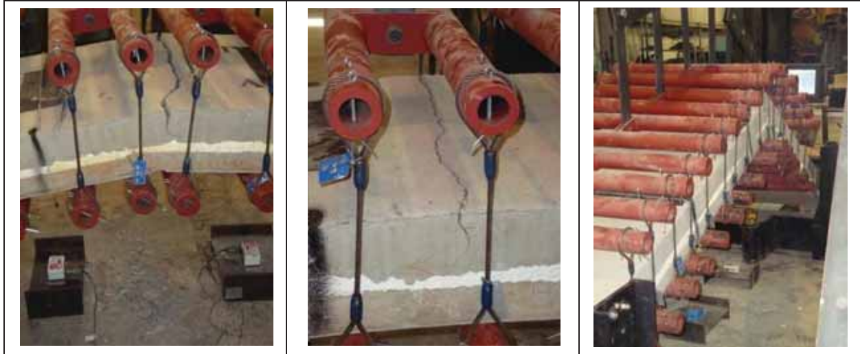
Figure 67. PCS2 Panel Response (A, B, C)
